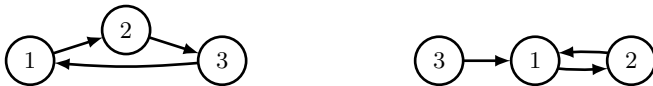
Fig. 1. Agent perception variations in static mapping when transferring from a two to a three agent task. An arrow from each agent denotes which other agent it is “aware” of.
